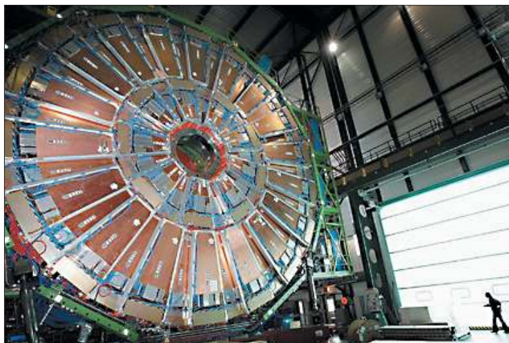
The world's largest superconducting solenoid magnet, preparing to take data at CERN's Large Hadron Collider (LHC) particle accelerator
